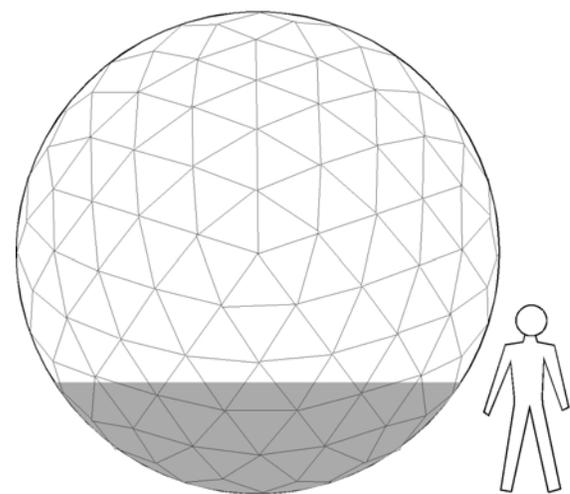
**Figure 4. Proposed experiment sphere.** *The sphere consists of a semi-transparent sphere with geodesic reinforcing struts. The darker gray region shows the approximate volume of the sphere that can be filled with solid material.*
